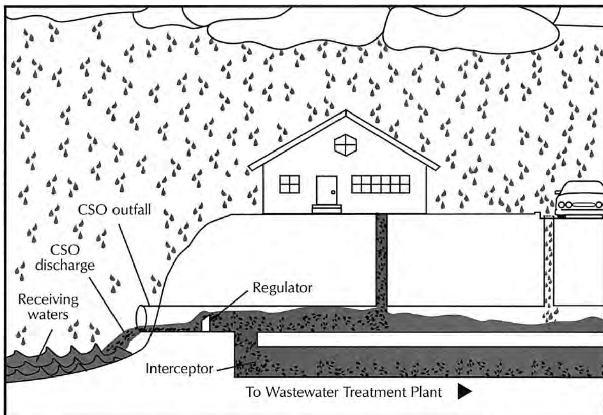
Figure 32.—Illustration of a typical combined sewer system. CSO = combined sewer overflow.
