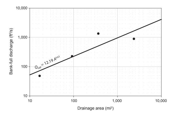
Figure 7.–Regional curve relating bank-full discharge (Qbkf) to drainage area for the Upper Menominee River drainage area in Michigan.
