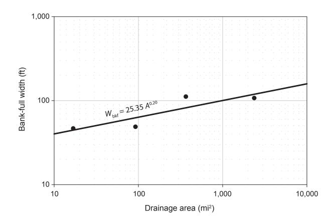
Figure 8.–Regional curve relating bank-full mean width (Wbkf) to drainage area for the Upper Menominee River drainage area in Michigan.
