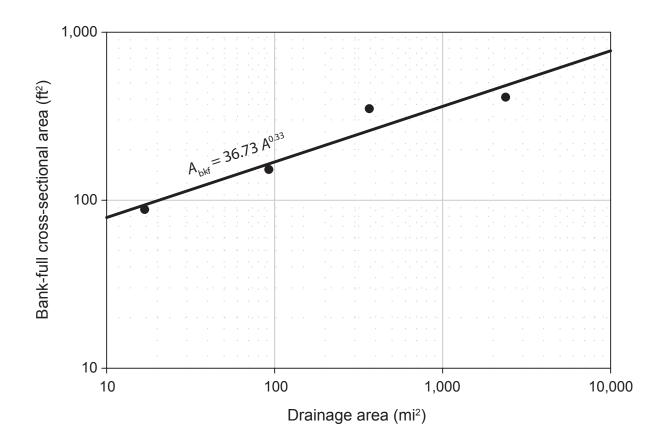
Figure 10.–Regional curve relating bank-full cross-sectional area (Abkf) to drainage area for the Upper Menominee River drainage area in Michigan.
