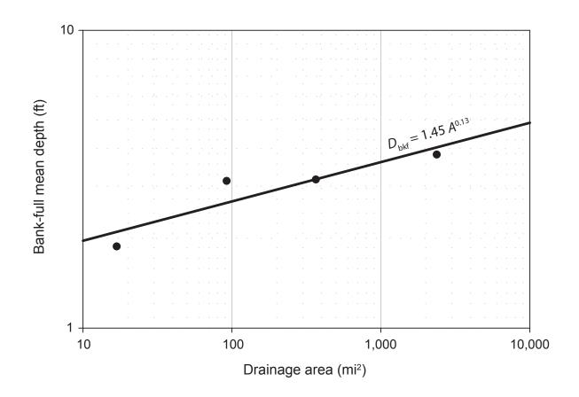
Figure 9.–Regional curve relating bank-full mean depth (Dbkf) to drainage area for the Upper Menominee River drainage area in Michigan.
