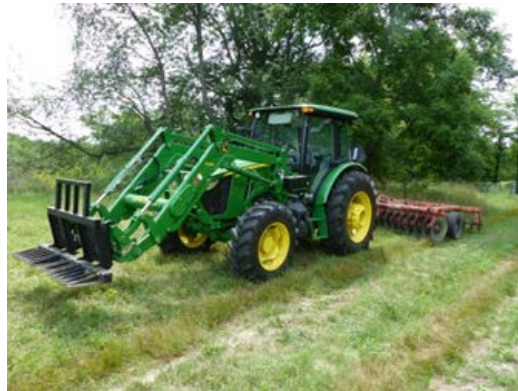
Tractor equipped with HedgeHog bar for removal of invasive shrubs. The disk is used to prepare a seedbed for food plots.
